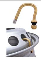
V53600 - Specialty Sprinter Valve. Works with Dodge, Freightliner and Mercedes Sprinters in Outer Rear Steel Wheels.
